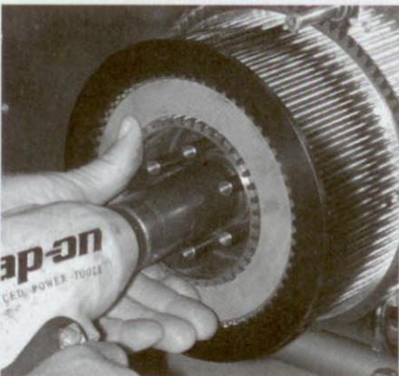
13 The supplied hub nut, which is a reverse threaded nut, can then be installed using a 1-1/8" deep socket and some red Loctite. Torque the nut to H-D spec.
