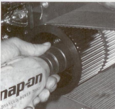
16 The Tech Cycle-supplied engine nut can now be installed, with some red Loctite on the threads, using a 1-5/16" socket. Torque the nut to H-D spec.
