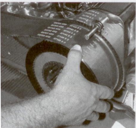
14 The Gates belt can now be slipped over the clutch assembly. Larry always installs the belt so you can read the lettering when alongside the bike.
