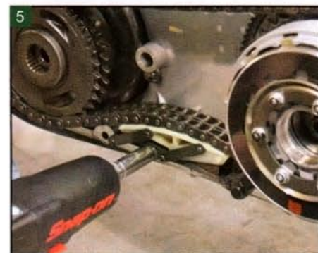
5 Remove the automatic primary chain adjuster mounting bolts and adjuster.
