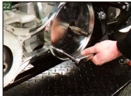
With the starter in place, the backside plate hardware can be tightened.
