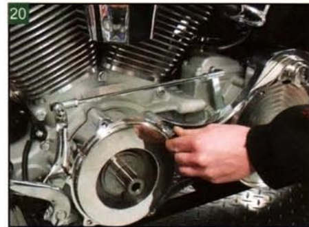
Start the backside plate mounting bolts, but do not tighten them now.
