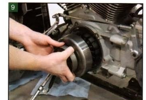
9 Carefully remove the stator rotor. This rotor needs to have the compensator assembly machined to fit.
