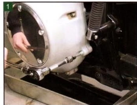
1 Start by draining the primary fluid and loosening the outer primary bolts.
