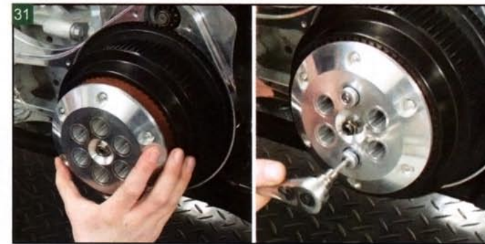
Line up the two dots and slide the pressure plate into the clutch basket. Install the springs, spring retainers, and cap screws into the pressure plate.
