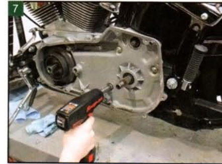
7 Loosen and remove the inner primary mounting bolts, and the two starter bolts from the other side of the bike.
