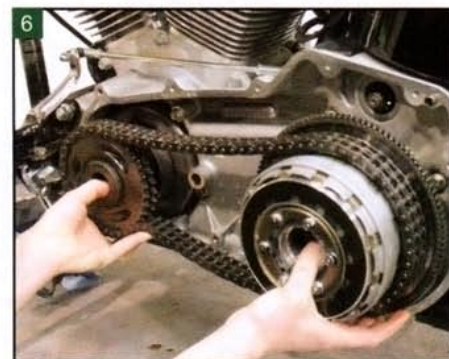
6 Then remove the primary chain assembly from the inner primary.
