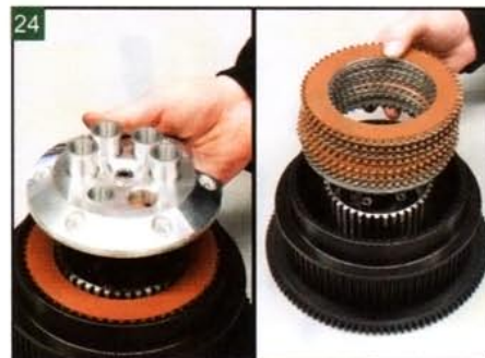
Then remove the pressure plate, spring cups, and clutch plates from the clutch hub.
