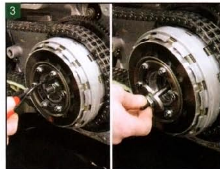
3 Use snap ring pliers to remove the retaining clip and remove the clutch adjustment plate.
