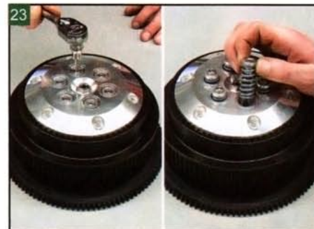
To install the clutch hub assembly, first loosen and remove the cap screws, spring retainers, and springs.
